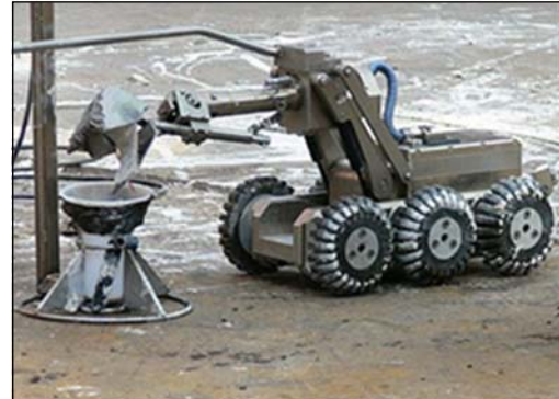
Current ORSS – General Electric Inspection Technology (GEIT) V3020-6310 Crawler and V9500-4001 Sample Scoop
