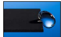
Water repelled by laser treated surface
