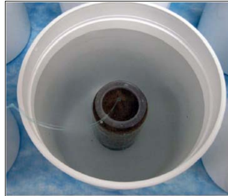
Monolith Leach Container During Leach Testing
