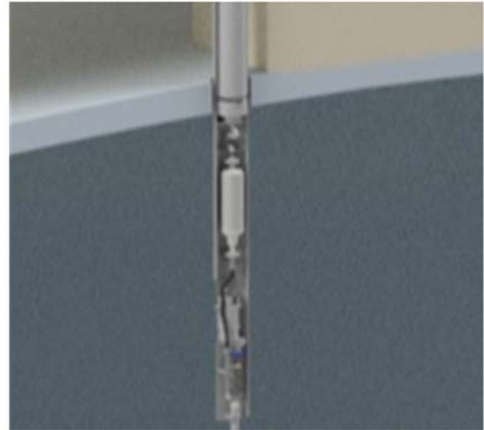
TBI 2 Waste Tank Pump
